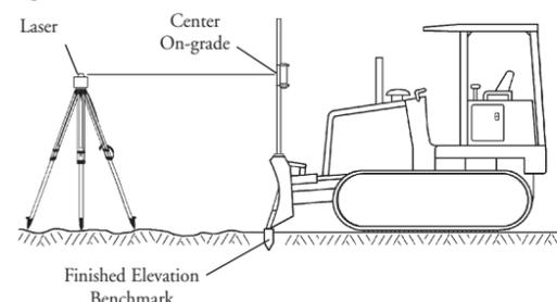
1. Position the machine so the blade can be set to the desired finished elevation (typically on a benchmark or hub stake).
