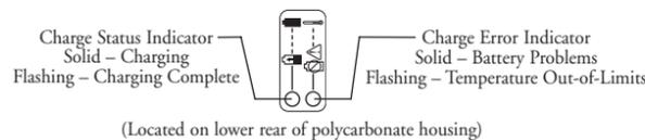
**Charge Status Indicator:** The LED remains solid when the batteries are charging. The LED flashes when the batteries are fully charged. When the batteries are charged, unplug the charger from the outlet, and remove the cannon adapter from the accessory connector.
