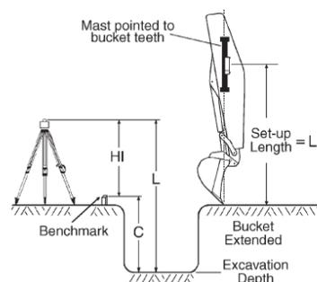
1. Set the laser up in an appropriate location for receiver visibility and efficient machine operation and turn it on.
