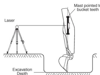
1. Position the machine and dig to the desired finished elevation.
